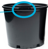
Increasing processing speed of current low melt flow PP resin results in a short shot.
